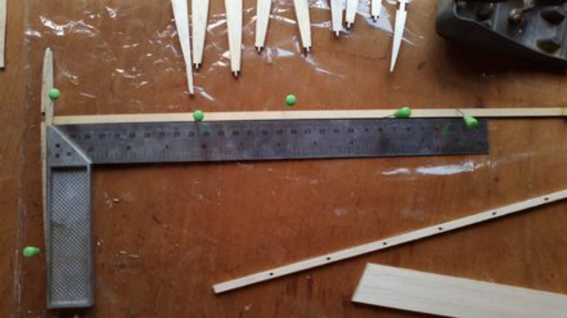
The „ear“ part of wing: start with first rib and ply support:
