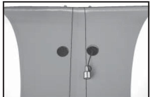
□ 3) Attach servo lead to the aileron servo. Attach the string to the servo lead and carefully thread it through the wing. Once you have thread the lead through the wing, remove the string so it can use for the other servo lead.
