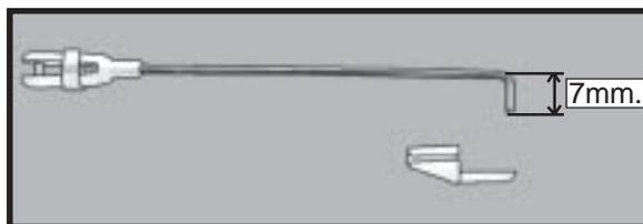
□ 9) Connect the linkage as shown and secure the control wire with a wire keeper.
